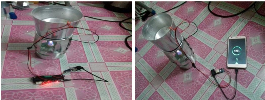
Fig.11. Use TEG to charge 3.7v Lithium battery to charge smartphone.
