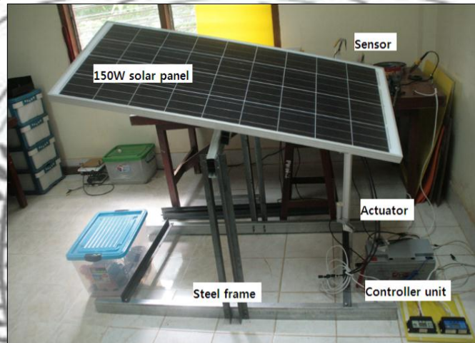
Fig. 1. 150W Solar photovoltaic module with a tracker developed in this study.
