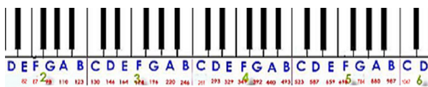
Figure 5: Musical notes from E2 - C6 is assign within the frequency range 82 Hz - 1047 Hz
