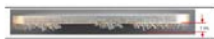
Figure 8 shows the result of cutting the fins W = 700w, f = 100Hz and CS = 500 mm / min
