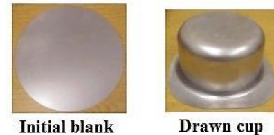
Figure 8 Initial blank size and drawn cups
